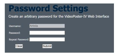
The new password must be entered twice to prevent the device from being inaccessible due to typing errors. Form data can be reset by clicking "Clear". By pressing "Submit" the new password will be activated and you will have to re-login on changing to any other page of the web frontend.
